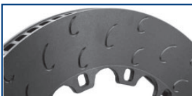
GC = 'J' Hook Design. As RC design but with outer grooves not running out to O/Diameter. Gives improved bite and debris clearance plus reduces distortion / vibration.
