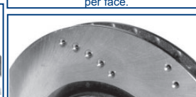
RD = Radius Drilled. (Cross drilled but with radius run out to reduce noise & improve life compared with standard cross drilling. Usually used on Road applications.
