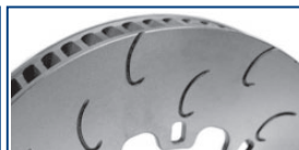
RA = 'J' Hook Design. Gives improved bite and debris clearance and reduces distortion / vibration, outer grooves run out to O/Diameter.
