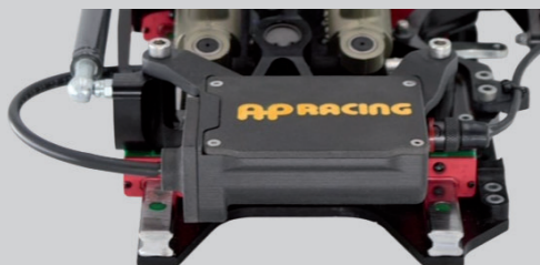
Close up of the AP Racing Brake Bias Adjuster with printed integral mounts
