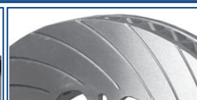
CR4, 8, 12, 24 = Curved Grooves. (Backward facing running out on O/D to clear debris. Only used on thick wall discs). The number specifies grooves per face.
