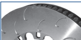
GA = 'J' Hook Design. Gives improved bite & debris clearance & reduces distortion / vibration, outer grooves do not run out to O/Diameter.
