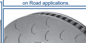
RC = 'J' Hook Design. As RA design but with 3 hooks across face. Gives improved bite and debris clearance, reduces distortion / vibration, outer grooves run out to O/Diameter.
