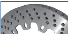
D & SD = Cross Drilled. (Drilled holes chamfered). Still preferred with some pad materials but can compromise disc life.
